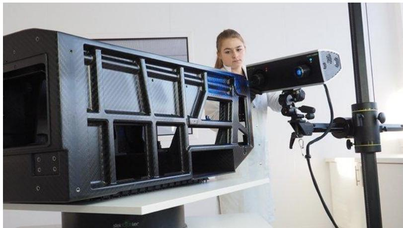
**Figure 3:** 3D-scanning of a structural component with complex geometry made of CFRP
