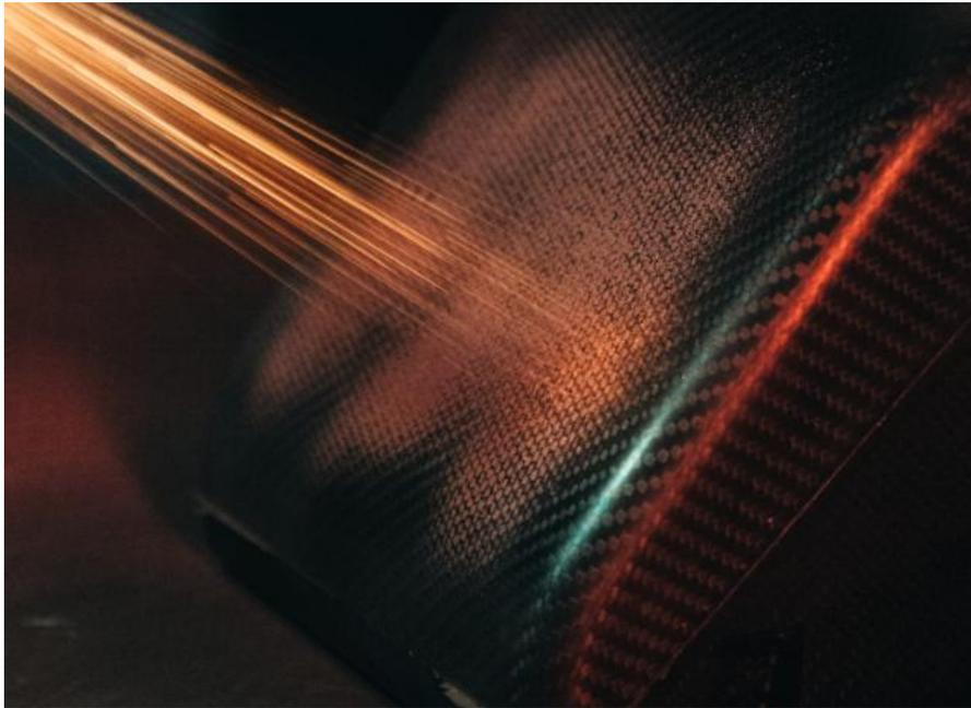
**Figure 5:** Applying an EMC protective layer to a carbon composite component by thermal spraying
