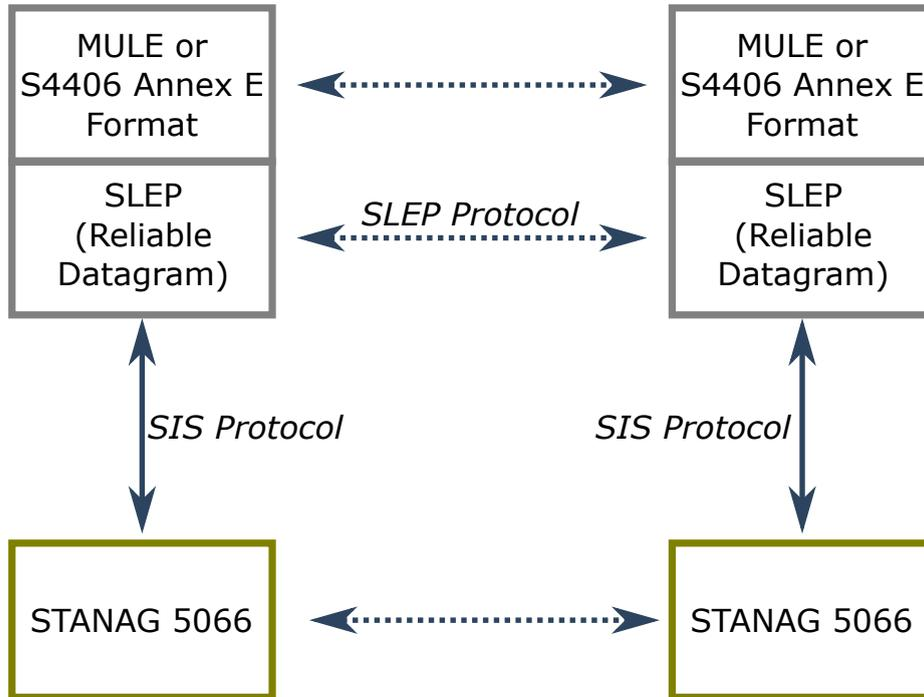
[SIS Layer Extension Protocol \(SLEP\) \(S5066-APP3\)](#) is an open standard that defines various services over STANAG 5066. The SLEP specification defines how to use SLEP for message transfer using the Reliable Datagram Service to transfer:
