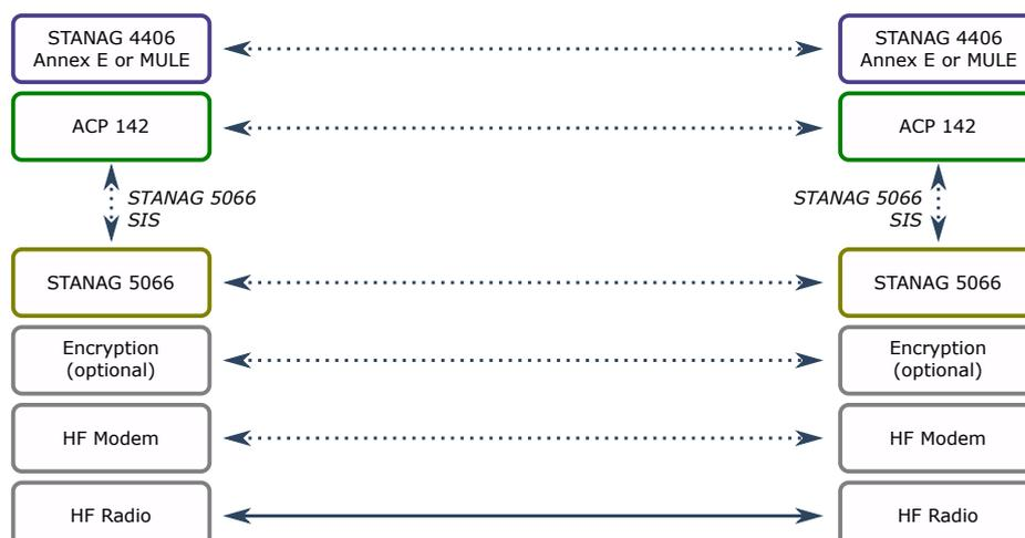
The diagram above shows the protocol stack used over HF Radio. STANAG 5066 Annex F standardizes ACP 142 operation over STANAG 5066. This protocol architecture has ACP 142 operating directly over STANAG 5066 using the Unreliable Datagram Oriented Protocol (UDOP). This direct mapping is optimized, and handles priority, as the priority of each ACP 142 packet is mapped on STANAG 5066 priority. This is important if multiple applications are operating over a single modem/radio.
