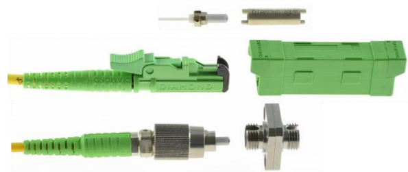
Figure 8. Examples of DMI (top), E-2000™ (middle) and FC (bottom) connectors with the corresponding mating adapters. DMI and FC connectors rely upon alignment keys based upon notch-slots combinations, while the E-2000™ relies upon its rectangular cross section.
