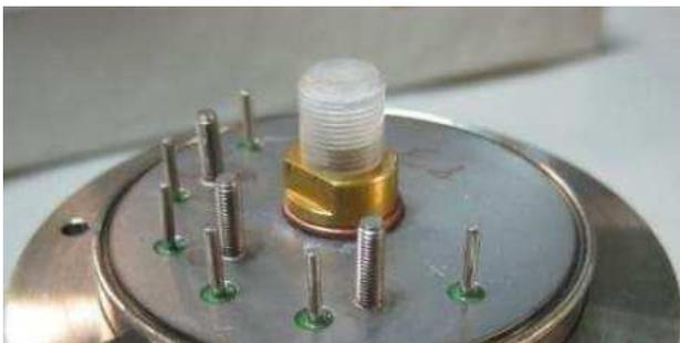
Figure 8: ISL laser igniter on header of a thermal battery
