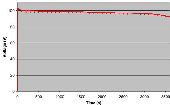
*Figure 9: discharge at 1.5kW continuous (60 minutes)*
