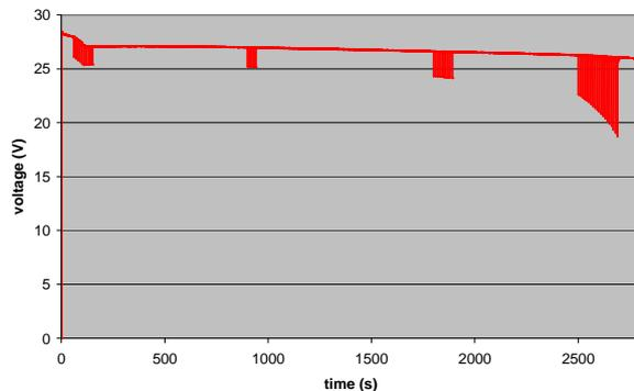
*Figure 10: discharge with 500W current pulses (45 minutes)*
