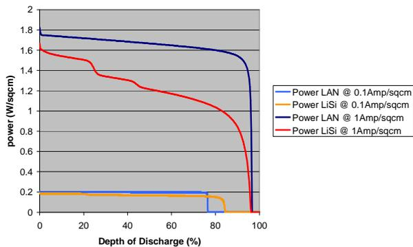
Figure 4 : comparison of power of LAN and LiSi cells @ 2 current densities (0.1 and 1 Amp/s)
