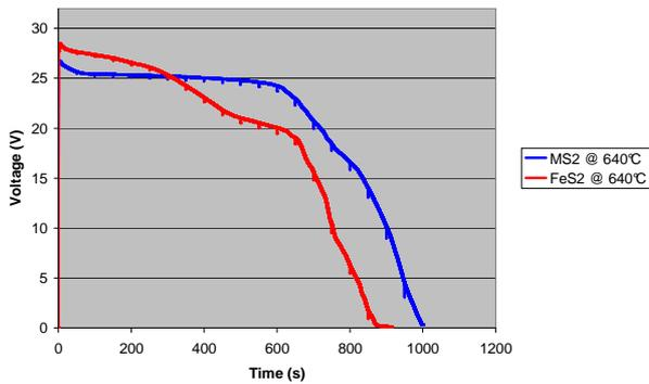
Figure 7: comparison  $FeS_2/MS_2$  @ very high cell temperature ( $640^\circ C$ )
