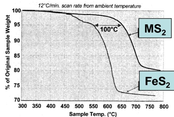
Figure 6 : Weight loss as a function of temperature
