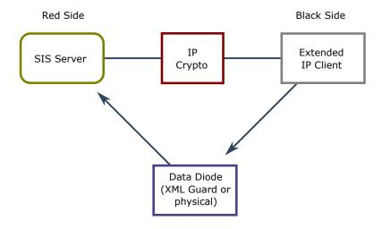
It is necessary to pass monitoring and control information from black to red side. This is achieved by a use of a data diode, which ensures that data only flows black to red. This might be a "physical" data diode that ensures unidirectional data transfer or it may be an XML Guard providing an application data diode service. Further details:
