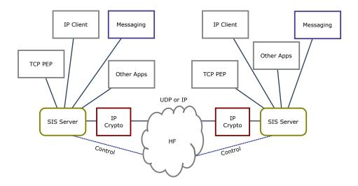
On the red side, a SIS server provides the STANAG 5066 SIS service to all applications. This looks exactly like standard STANAG 5066 to all of the applications. This makes the service completely transparent to all the HF applications.
