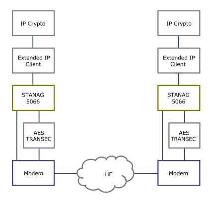
The black side architecture needs to transfer IP packets being sent through the IP Crypto. This is achieved using standard STANAG 5066 using STANAG 5066 Annex F.12 IP Client to do the IP transfer. Key points on the black side architecture:
