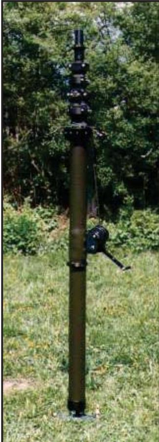
The mast is basically composed of telescopic sections made of **composite material ("fiberglass")** by use the process of "pultrusion". By use of that technology all the fibres are placed longitudinally along the section enable excellent stability with high degree of elasticity. Certain fiberglass layer is also wounded radially during the pultrusion process enables high degree of radial hardness. The masts STV meet environmental requirements in accordance with **MIL-STD-810**.
