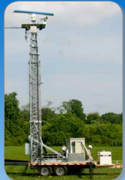
Pneumatic Mast with Remote Locking System
