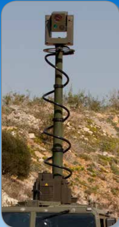
Pneumatic Mast with Remote Locking System
