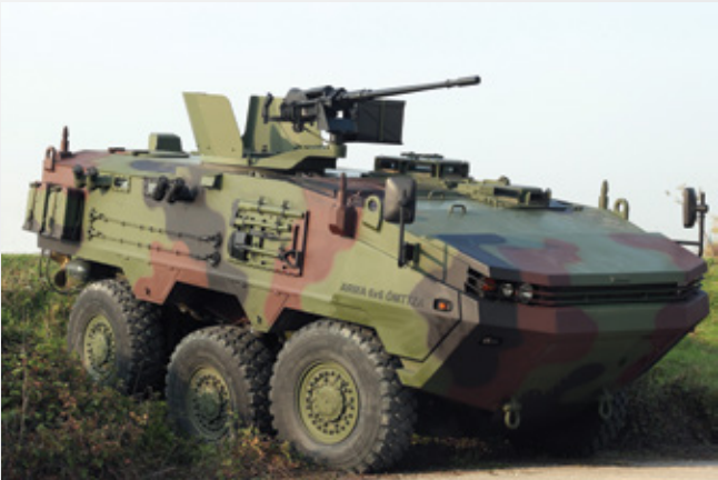
ARMA PERSONNEL CARRIER WITH OPEN CUPOLA (20 MM CANNON)
