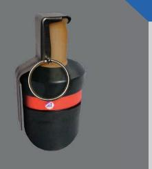
Sound and light grenade with irritant (CS/CN) one and multi-chamber with different effects is equipped with ADQ-01 fuse. The body is made of polymer material with low glass transition and blistering temperature that excludes fragments formation during grenade usage. Typically the body material fragments into straps and bands of random shape with no lethal effect during pyrotechnical charge explosion.
