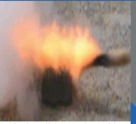
Smoke-puff charge is designed for staff training. It imitates grenade explosion. There is an incendiary knot on the end of a cord which is initiated by the flame or granting method.
