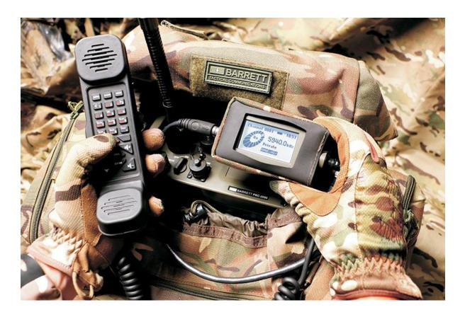
Barrett Communications offers the PRC-2090 as a high-frequency (HF) radio solution for rapidly changing operational environments.
