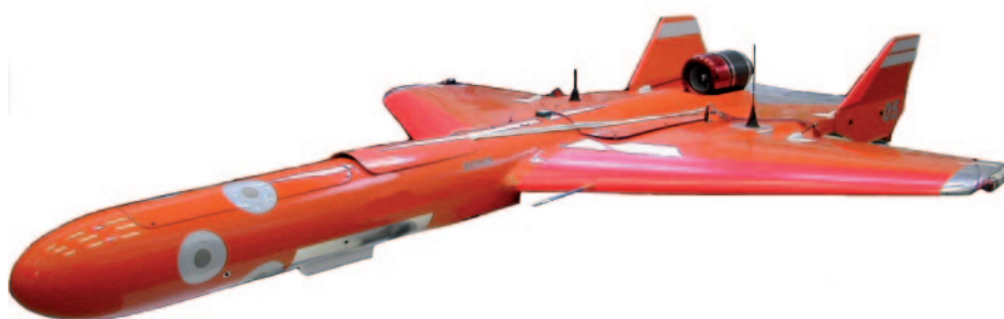
MDI AS-135/12U installed in the SCRAB TARGET
