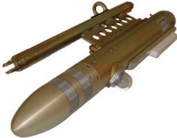
MDI AS-131/12U EQUIPPED WITH A UPLINK CONTROLLED HALOGEN LAMP FOR NIGHT FIRINGS
